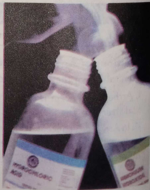
Fig. 10.6 Hydrochloric acid gas combines with ammonia gas resulting in white smoke of solid ammonium chloride.
