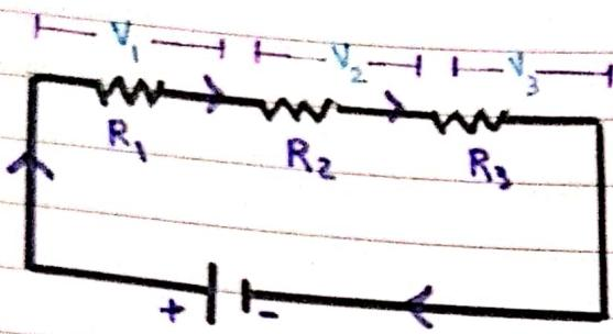
Resistors are connected end to end
