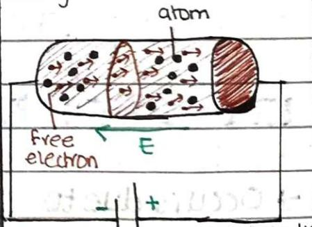
Drift of free ēs through conductor
