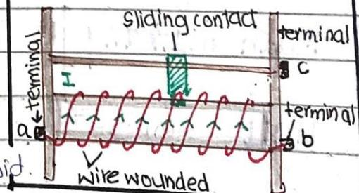
→ **Function** Rheostat is a current controlling device. It acts as a potential divider in the circuit. If the fixed terminals are connected in the circuit it acts as a fixed resistor. If the variable terminal along with one fixed terminal are connected, it acts as variable resistor.
