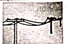
Wires on electric poles are given some sag to prevent breaking in winter
