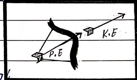
Conversion into K.E:- When arrow is shot then its stored elastic potential energy converts into its Kinetic energy of arrow due to which arrow moves in the forward direction.
