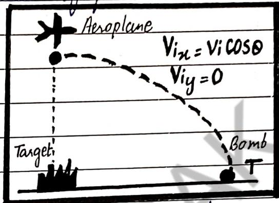
→ The bomb misses the target if it's dropped vertically above the target because it moves like a projectile.
