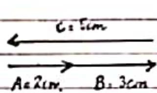
$\rightarrow$  It is clear that sum of the vectors is zero because the head of the last vector  $\vec{C}$  coincides with the tail of first vector  $\vec{A}$ .
