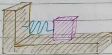
(a) Mass spring system is at rest. No force is applied on the mass. It has covered zero displacement
