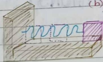
(b) Force F is applied to displace the body to point 'A'. After reaching point 'A' restoring force pulls the body back to 'O' but due to inertia, mass moves to point 'B' compressing the spring. This way vibratory motion proceeds.
